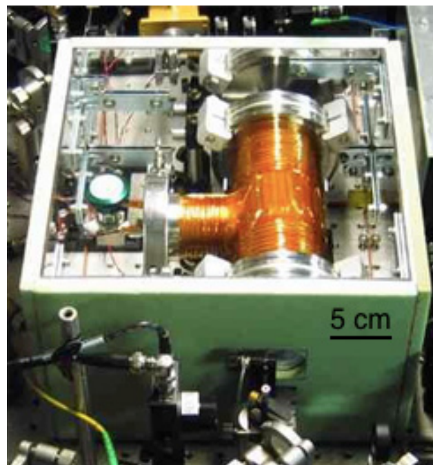
Figure 3.5: Vacuum housing and outer acoustic shielding box for the 741 nm optical cavity. Cover of the shielding box is removed for the photograph.
