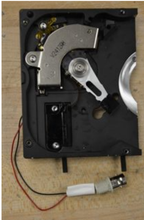
Figure 2.6: Picture of a beam shutter made from a hard drive. A hole is drilled in the casing to allow the beam to pass. A black metal piece is glued to the read/write head and is used to shutter the beam. The black metal was cut out of a Coca-Cola Zero can.
